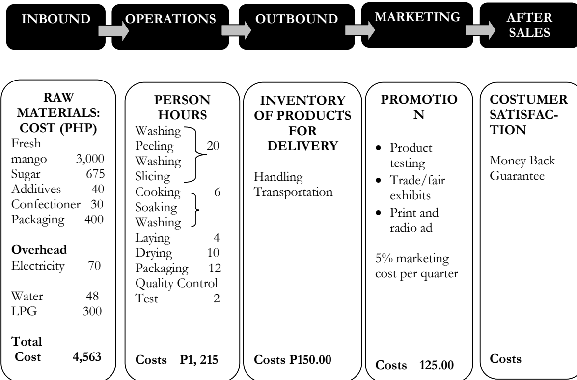
Figure 35. Process Flow for Mango Processing with Costing
